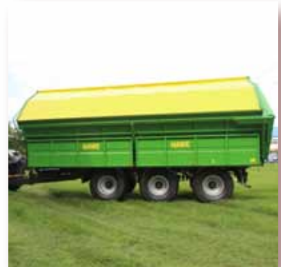
Dumper trailer bodies in different models from 22 to 44 cubic metres.
