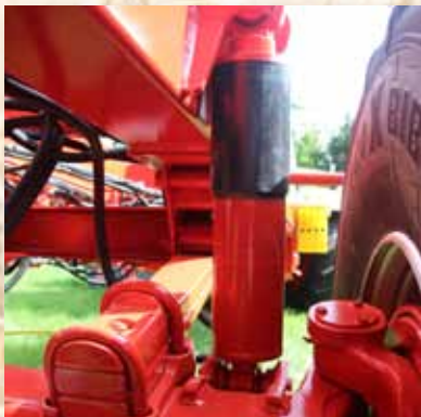
Running gear with hydraulic suspension.
