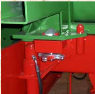
Twist-Lock locking system with parking stand holder.
