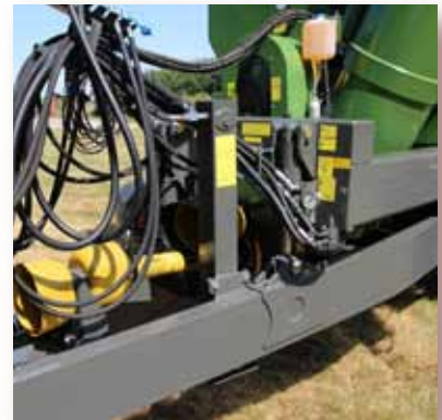
Hydraulic parking stand and hydraulic drawbar suspension.
