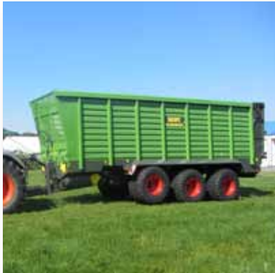
Silage transport trailer bodies from 38 to 50 cubic metres capacity.
