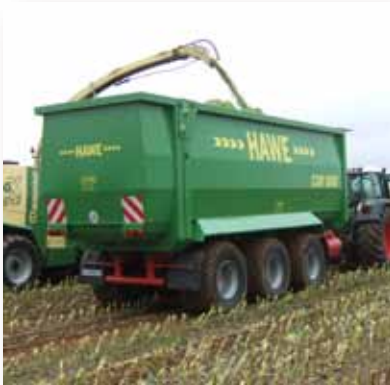
Cargo push-off trailer body with 40 or 50 cubic metres capacity.
