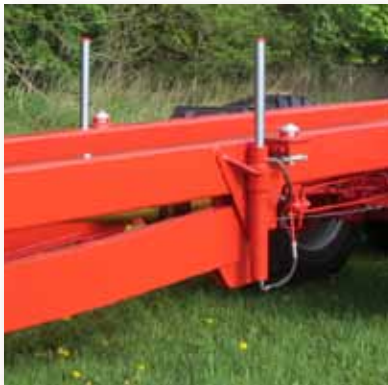
Lifting rams to remove and install the different bodies.
