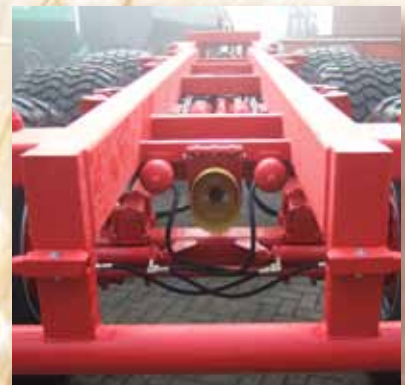
Tridem running gear with PTO shaft for the body drives as standard equipment.
