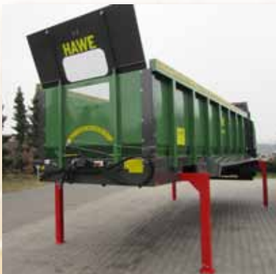
Universal and manure spreader bodies, from 15 to 23 cubic metres.
