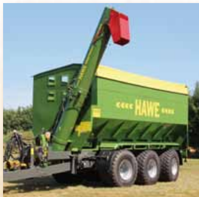
Field transfer trailer bodies for grain, from 25 to 38 cubic metres.
