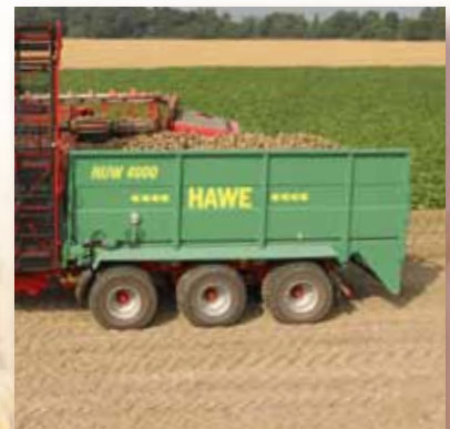
Beet transfer trailer bodies, capacity of 27 (tandem) and 40 (tridem) cubic metres.
