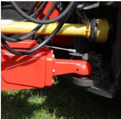
The positive steering system is controlled by a Bowden cable.
