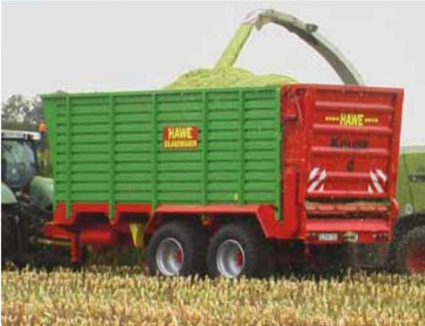
make the silage transport trailer easy to tow and only exert slight pressure, protecting the soil.
