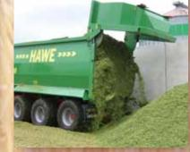
HAWE CSW 5000 with tridem running gear and parabolic suspension with self-steering for the first and third axle. Positive steering is available as an option.
