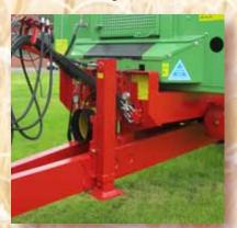
Hydraulic parking stand and hydraulic drawbar suspension.
