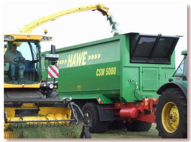
HAWE push-off trailers feature a strongly-built sheet steel body which is capable of withstanding high stresses. The bulkhead is operated by its own on-board hydraulics which are actuated by an electrohydraulic remote control system.
