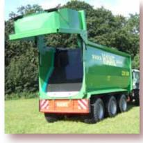
The bulkhead is operated by a multi-stage telescopic ram. The HAWE CSW experiences very little wear because moving parts are reduced to a minimum.
