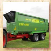
HAWE CSW 4000 with tandem running gear and hydraulic suspension, incl. lift axle and self-steering.
